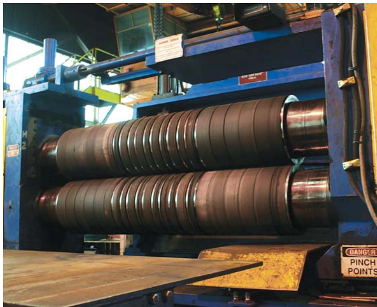
Ratner's slitter works as a partner to the company's cut-to-length lines, cut-edging coils for customers.
